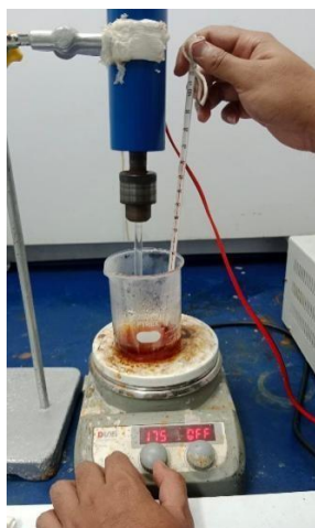
Figure 1. Mixing process of \text{FeCl}_3 \cdot 6\text{H}_2\text{O} and \text{FeSO}_4 \cdot 7\text{H}_2\text{O}
