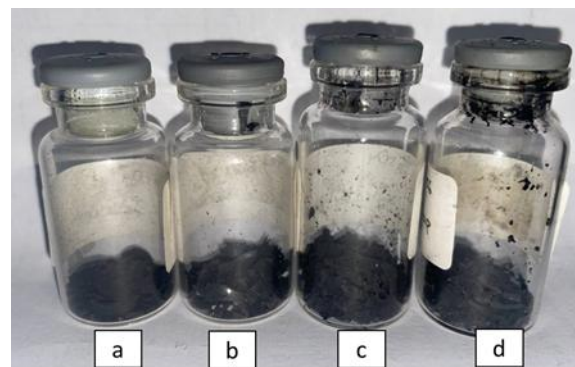
Figure 2. Visual characterization of \text{Fe}_3\text{O}_4 at (a) 70^\circ\text{C} in an open system, (b) 70^\circ\text{C} in a closed system, (c) 90^\circ\text{C} in an open system, and (d) 90^\circ\text{C} in a closed system
