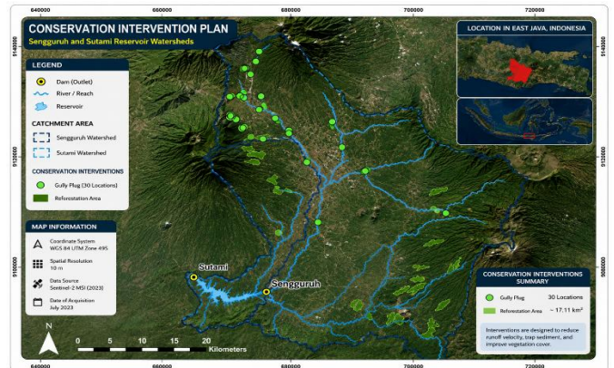
Fig. 6. Spatial distribution of proposed soil and water conservation interventions in the Sengguruh and Sutami reservoir watersheds.
