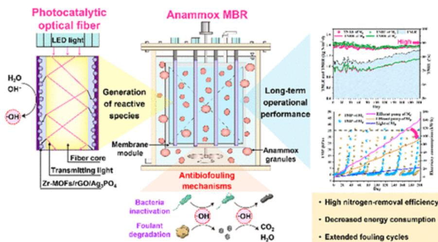
**Fig. 3.** The Zr/MOFs/rGO/Ag<sub>3</sub>PO<sub>4</sub> on POF membrane for Anammox MBR [51] (Reprinted with permission from [6]. Copyright 2023 American Chemical Society)
