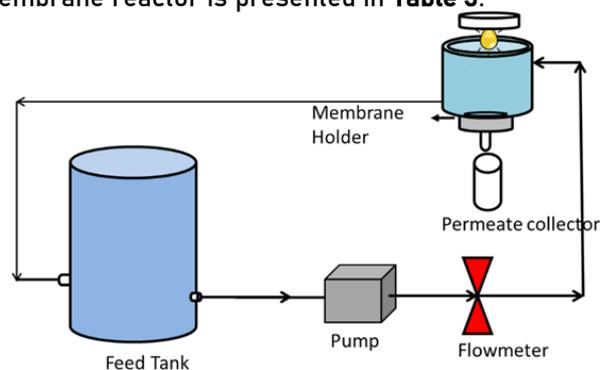
Fig. 2. Configuration of Cross-flow PM reactor
