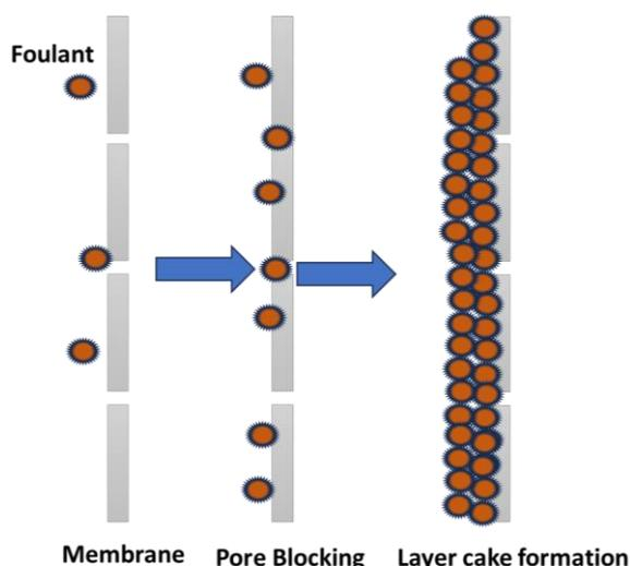
Fig. 1. Membrane fouling mechanism
