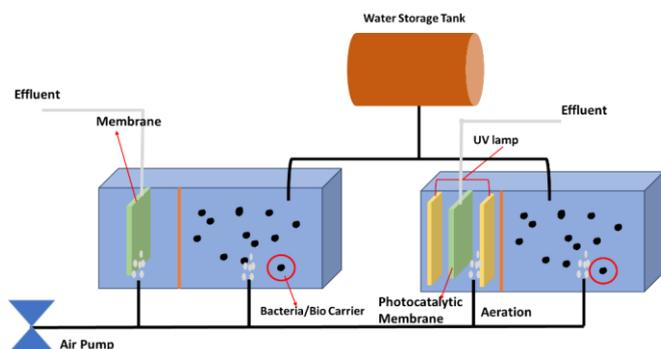
Fig. 4. Membrane Bioreactor configuration with nanomaterial-modified membrane.
