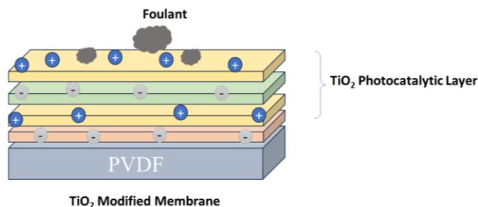
Fig. 5. TiO<sub>2</sub>/PVDF-modified membrane configuration
