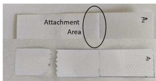
**Fig. 4.** Paper before (top) and after (bottom) tensile test.
