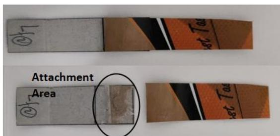
Fig. 6. Cardboard before (top) and after (bottom) tensile test.
