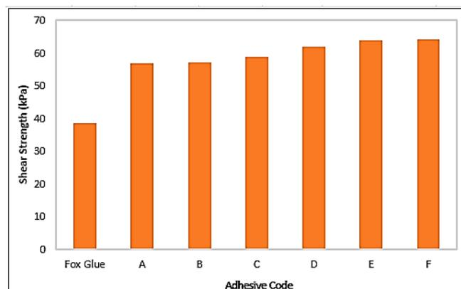
Fig. 7. Shear strength graph of various adhesives with cardboard material.
