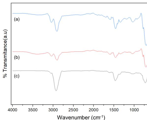
**Fig. 1.** Infrared spectra of (a) adhesive sample; (b) polystyrene waste; (c) gasoline.
