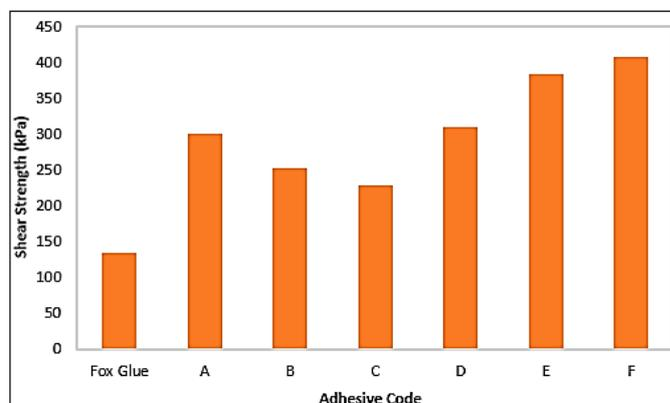
Fig. 9. Shear strength graph of various adhesives with wood material.
