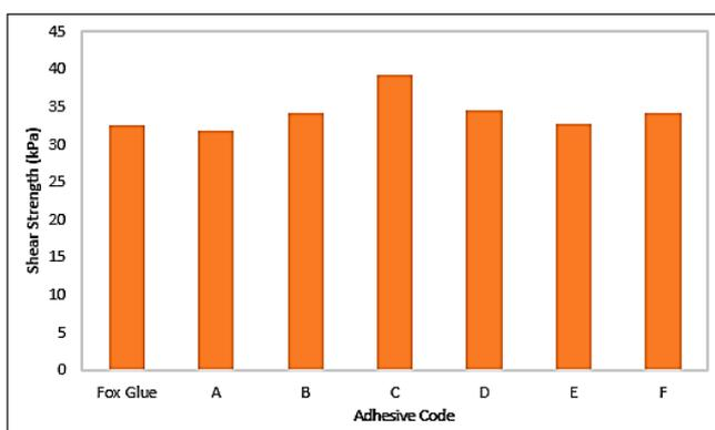
Fig. 5. Shear strength graph of various adhesives with paper material.
