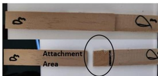
Fig. 8. Wood before (top) and after (bottom) tensile test
